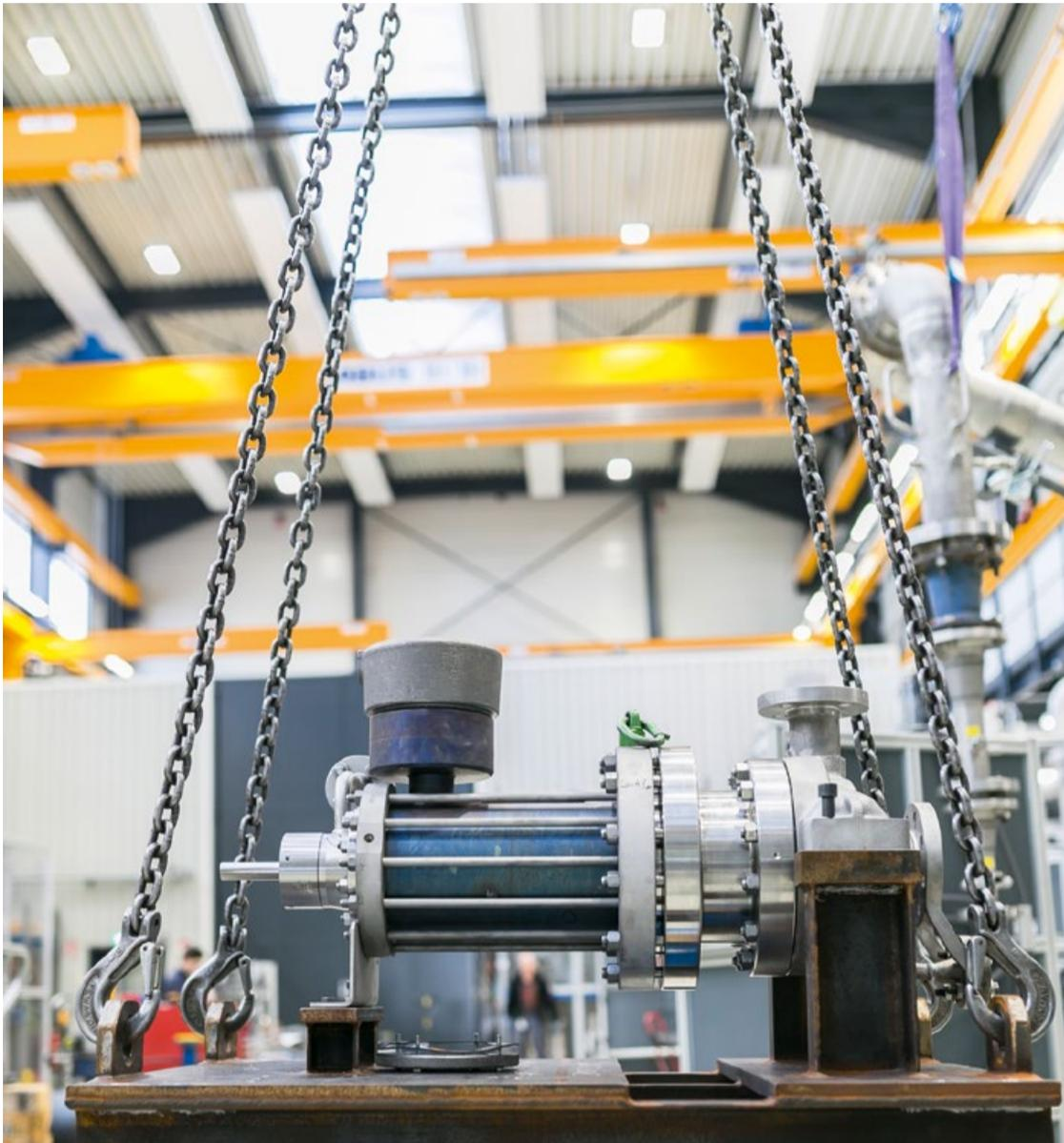
A canned motor pump according to API 685 in preparation at the new test bench
