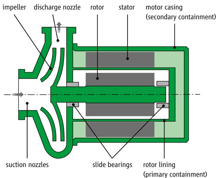
Diagram of a multistage canned motor pump
