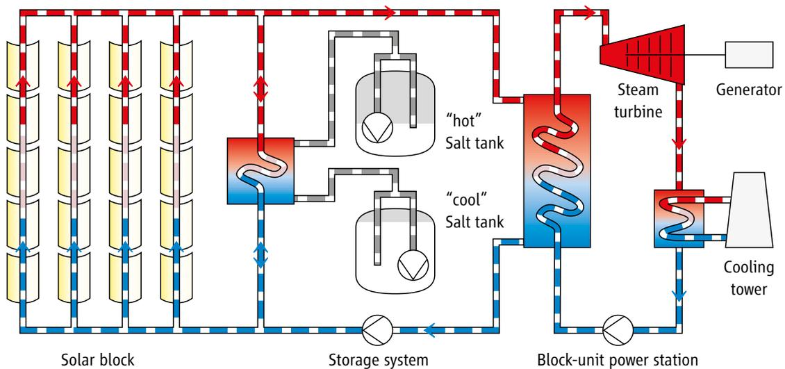
Diagram of a DISS pilot plant
